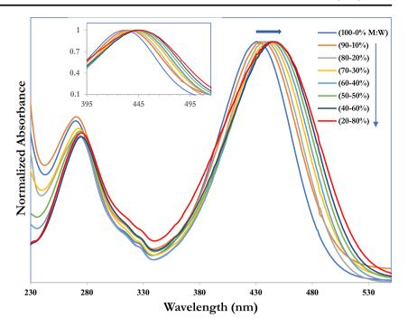
energy with substantial drop in intensity (cf. Figures 1a and b). The explanation for this, is that  $S_0 \rightarrow S_1$  is a  $^1(\pi,\pi^*)$  in nature, with charge transfer from dimethylaniline to the C=O moiety, which will facilitate solute—solvent interaction through H-bonding, causing stabilization to this state.
