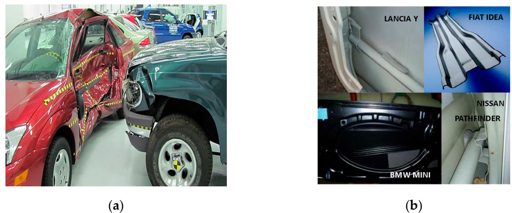
Figure 1. (a) Example of side impact between vehicles (source of image: Brady Holt, CC BY 3.0, via Wikimedia Commons). (b) Example of door intrusion beams/side impact beams (source of image: Strano. m, CC BY 3.0, via Wikimedia Commons).
