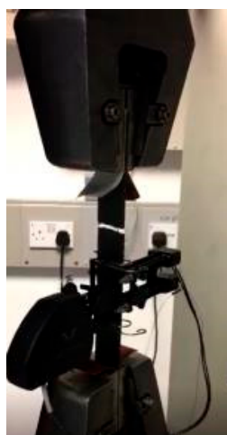
Figure 4. Composite samples under quasi-static loading with strain transducers.
