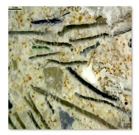
Fig. 10: Mortar based gypsm + 25% of PET particles
