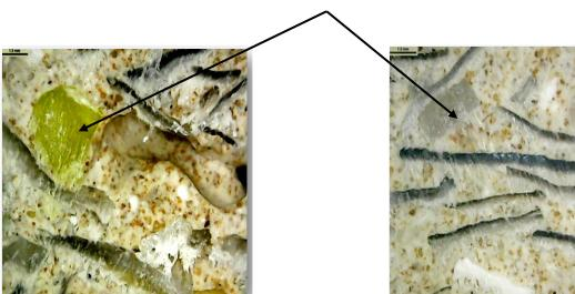
Fig. 8: Mortar based gypsm + 15% of PET particles
