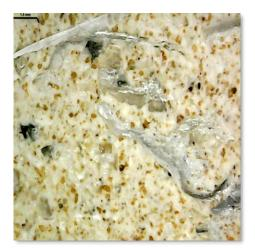
Fig. 6: Mortar based gypsm + 5% of PET particles
