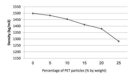
Fig. 2: Variation of the density of gypsum mortar according to the percentage by weight of PET particles
