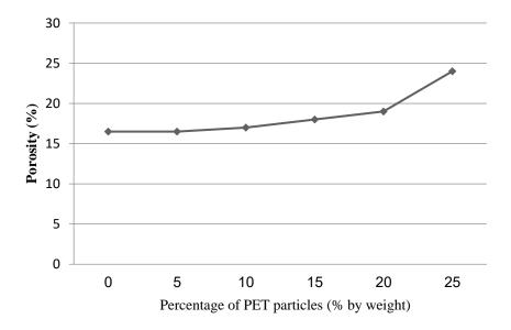
Fig. 3: Variation of the porosity of gypsum mortar according to the percentage by weight of PET particles
