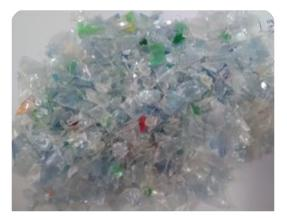
Fig. 1: Polyethylene terephthalate (PET) particles of plastic recycled bottles
