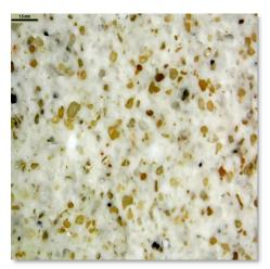
Fig. 5: Mortar based gypsm Matrix
