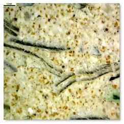
**Fig. 7:** Mortar based gypsm + 10%of PET particles
