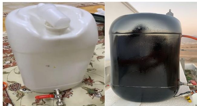
Fig. 1: Reactor arrangement (HDPE container, 30 litres size) with stainless steel valve (bottom) sampling outlet, gas outlet (top)
