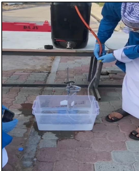
Fig. 2: Water displacement method setup for measuring gas volume
