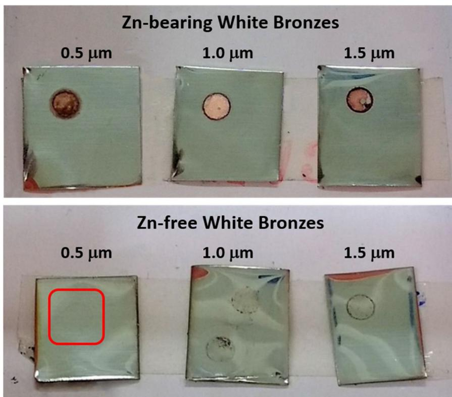
Fig. 10. Zn-bearing (top row) and Zn-free (bottom row) samples after polarisation cycles; the red square indicates an almost-invisible corrosion mark for the 0.5μm Zn-free sample. (For interpretation of the references to colour in this figure legend, the reader is referred to the web version of this article.)
