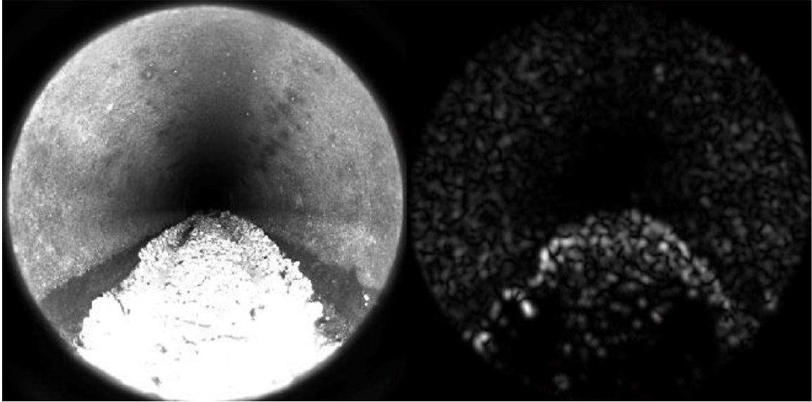
Figure 30, CCTV Camera Footage while Testing Using Gabor Filter
