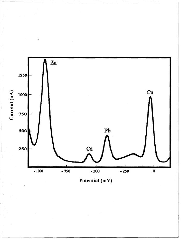
Figure 1: Typical voltammogram of wet digested khat (300 mg) after dilution to 250ml. Deposition potential -1100 mV; deposition time 120s for Cd, Pb and 30s for Cu. Zn; scan rate 6 mV/s; pulse amplitude 50 mV.
