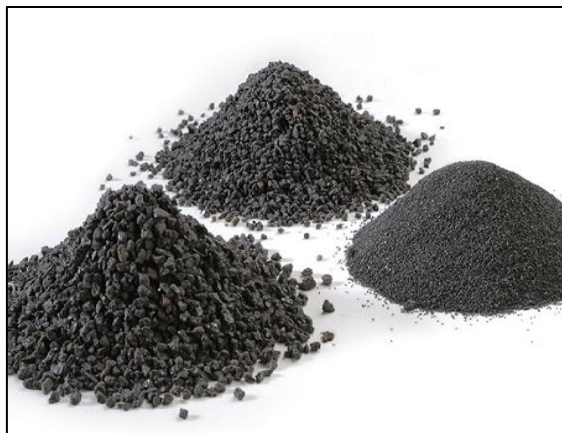
Figure 15: Steel slag of different particle size as it was grinded to 75 and 425 nm
