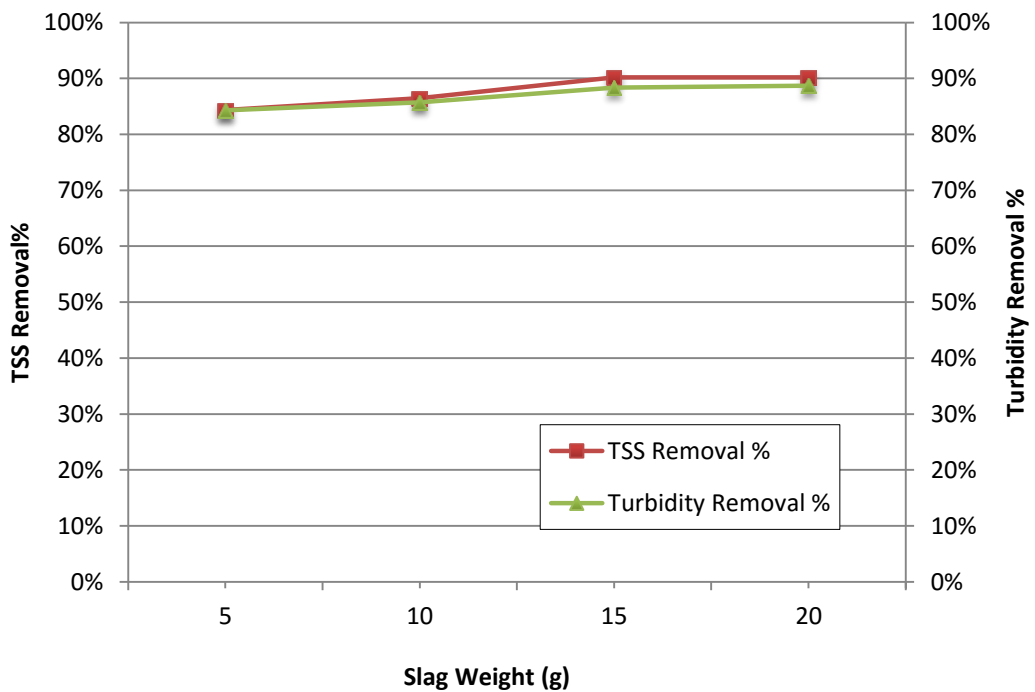
Figure 29: Turbidity (NTU) and TSS (mg/l) removal % of different weights of 75 nm steel slag over 40 minutes
