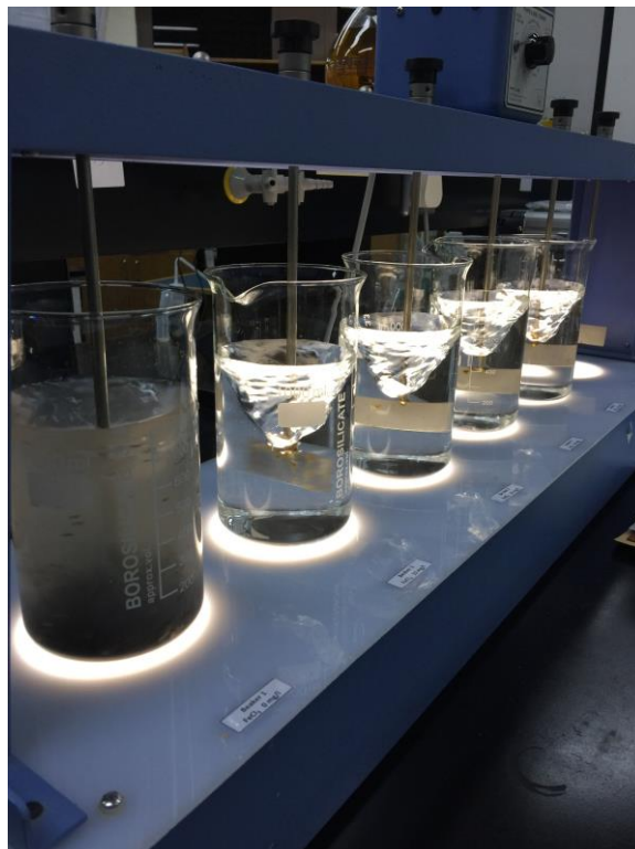
Figure 18: Jar test apparatus used for the treatment of dewatered construction water samples
