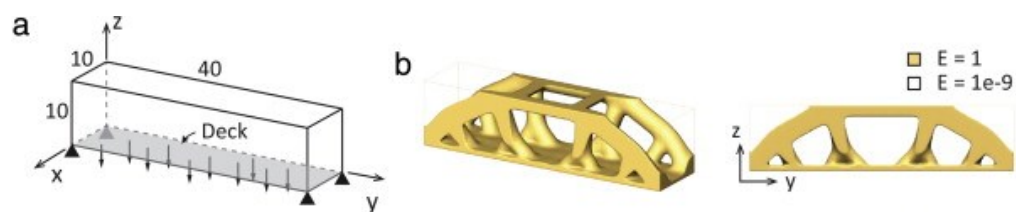
Figure 9 - Topology Optimization Example to a simple beam (Park & Sutradhar, 2015)
