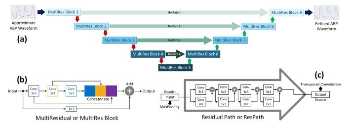
**Figure 3.** (a) Refinement Network. The PPG2ABP pipeline utilizes a 1D-MultiResUNet Network consisting of (b) MultiResidual Blocks and (c) Residual Paths to refine the approximate waveform constructed by the Approximation Network.
