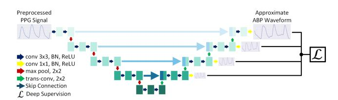
**Figure 2.** Approximation Network. PPG2ABP employs the Approximation Network to derive an approximate ABP waveform from the preprocessed PPG signal. The network is a deeply supervised one-dimensional U-Net, designed to solve regression problems.
