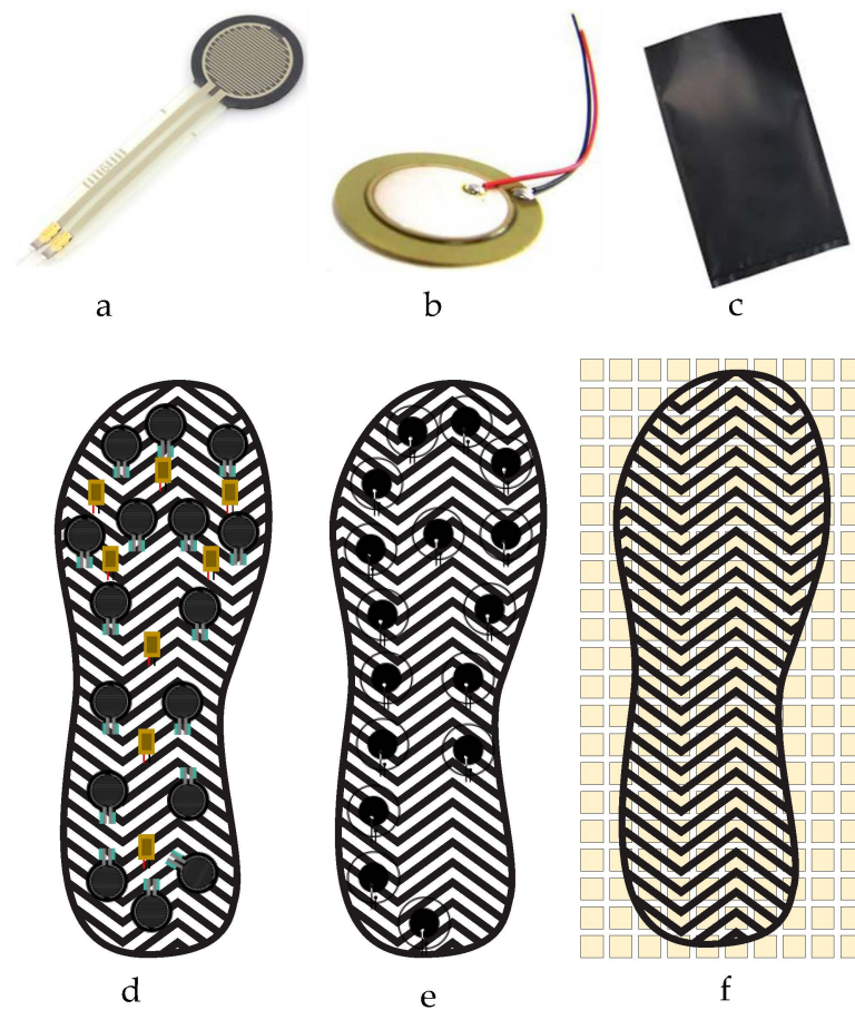
Figure 2. Three different electronic pressure sensors and their placements: (a) FSR, (b) Piezo-electric, (c) Velostat sensors; and (d) FSRs, (e) Piezoelectric Sensors and (f) the Velostat Sheet (with switching matrix) on an Insole.
