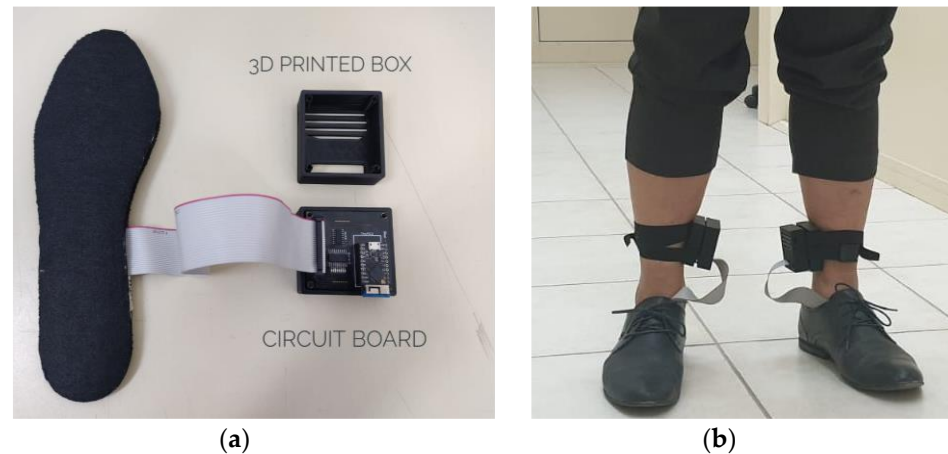
Figure 8. (a) Complete setup comprising of the insole, 3D printed box and the printed circuit board, (b) Setup placed on the human leg.
