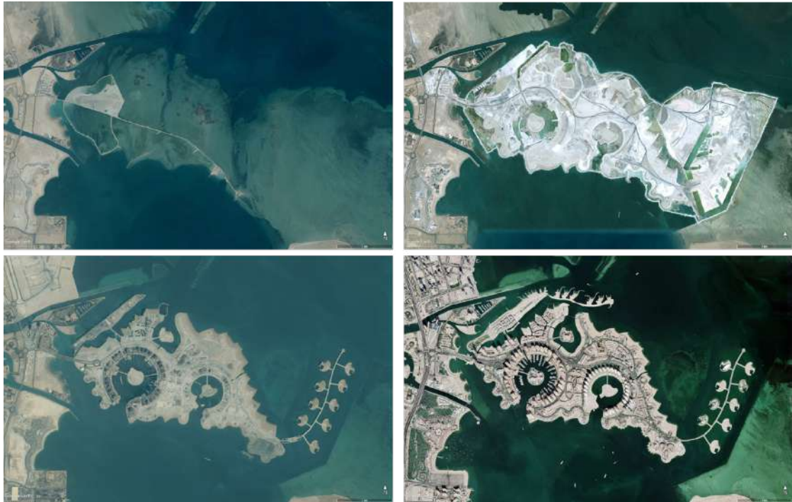
Figure 55. The Pearl-Qatar land reclamation process (top, left-to-right) 2004 and 2006 and (bottom, left-to-right) 2008 and 2022. Source: Google Earth.
