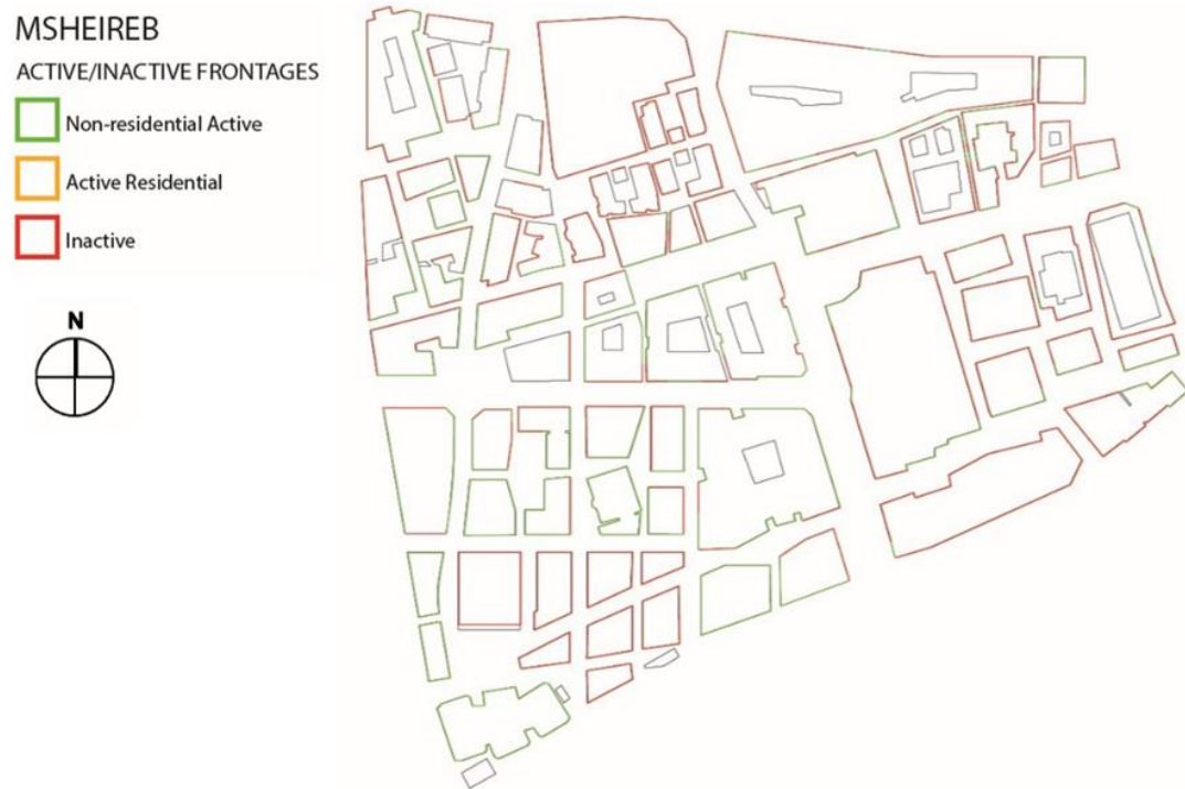
Figure 37. The map of active/inactive frontages. The green shows non-active residential frontages, while the red shows inactive ones. Source: Amleh et al, 2023/QUCG-CENG-22/23-472.
