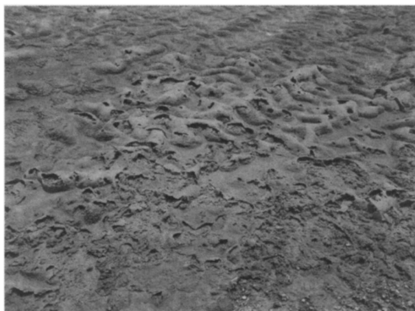
Figure 1. Surface crust of the Dukhan sabkha showing the friable nature of the mixture of sand, carbonates and halite.
