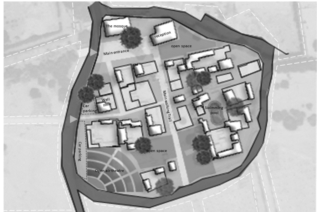
Figure 10. New proposed master plan layout and spatial modification for the village of Tinbak.
