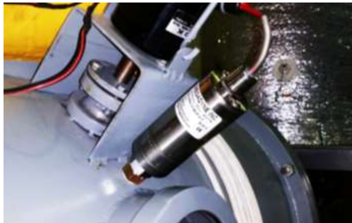
Figure 24 - Pressure transducer mounting
