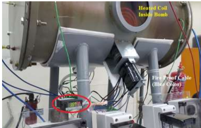
Figure 30 - Installation of heating coils
