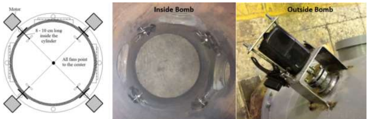
Figure 16 - Fans design and installation
