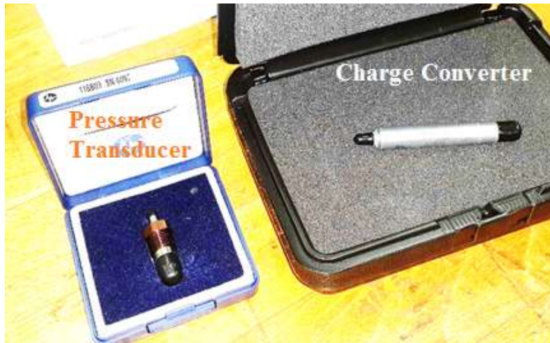
Figure 26 - PCB pressure transducer and PCB charge converter
