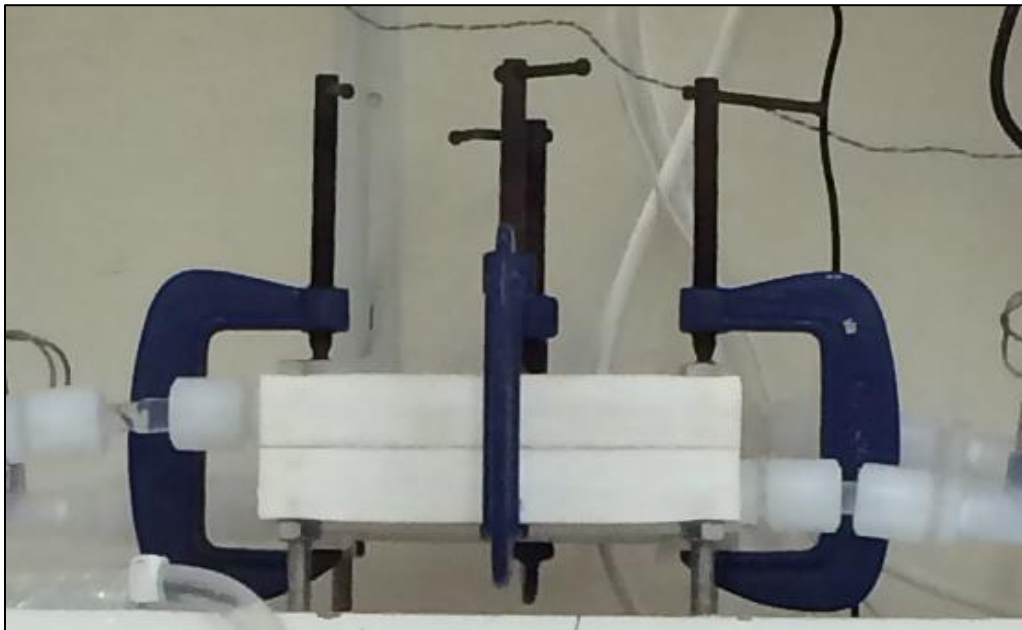
Figure 29: The DCMD Cell Used in the MD Unit with Clamping
