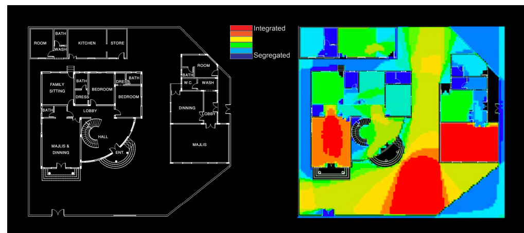
Figure 7. (left) Plan of ground floor level and (right) visibility graph analysis overlay for Villa #3 (Source: Authors).
