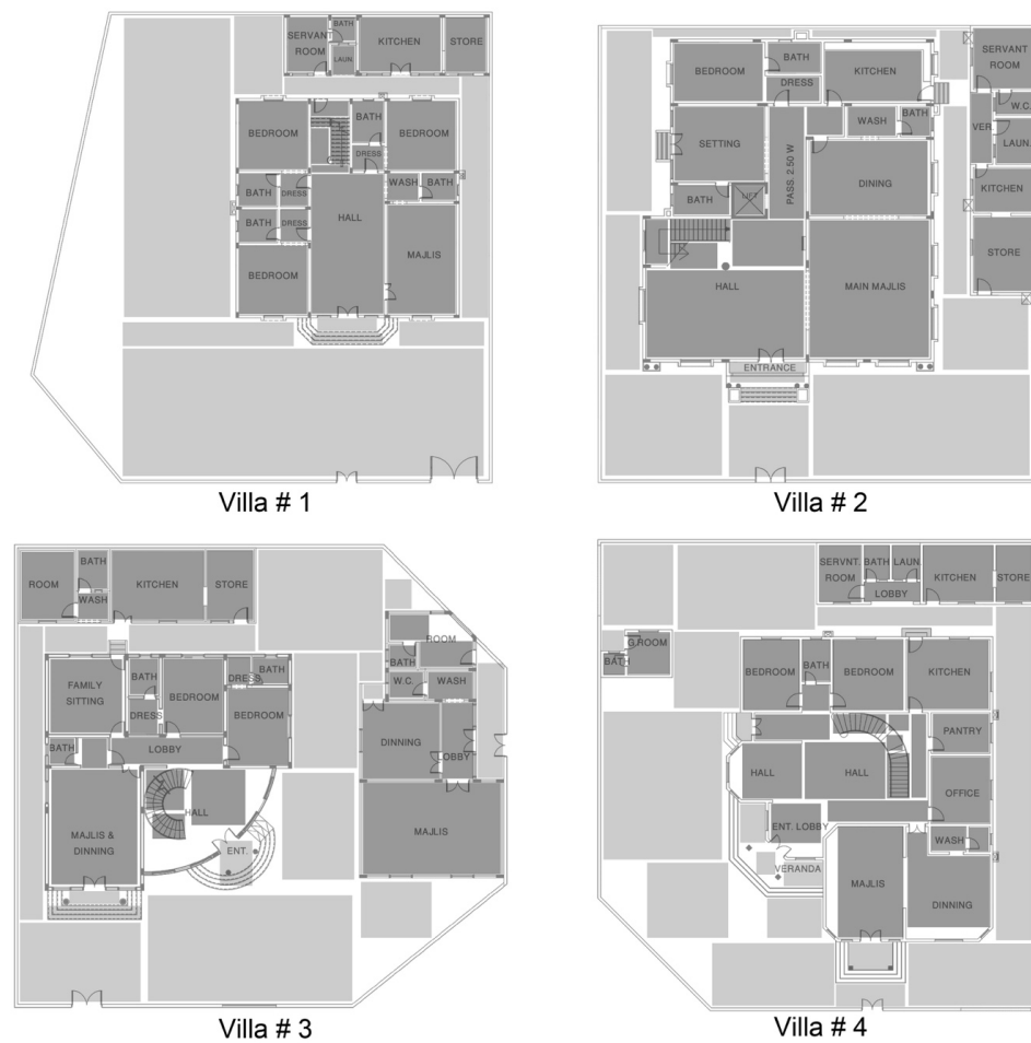
Figure 3. Convex spaces for the ground floor plans of the four contemporary villas are dark grey for interior spaces and light grey for exterior spaces (Source: Author).
