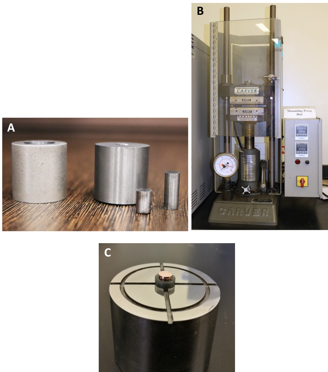
Figure 3.6 (A) From left to right; eject tool, die, and punches. (B) Carver mounting press. (C) Steel die along with the glass piece and \sim 1 mm sample disk above them.
