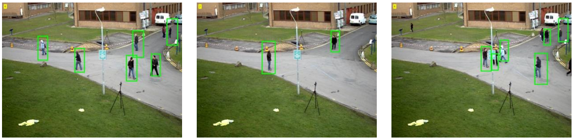
Figure 4.5. Examples of pedestrian detections using the proposed Faster R-CNN where the size of the bounding boxes is larger than the pedestrians
