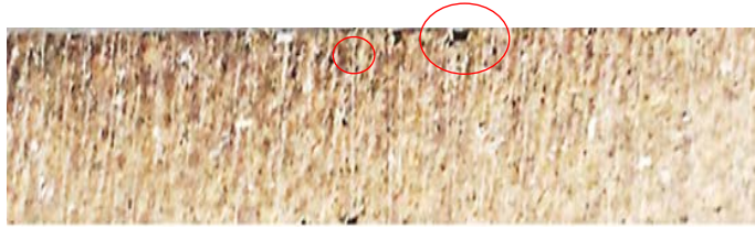
Figure 16: Cross-sectional image of the of wood polypropylene particulate bio composite panels.
