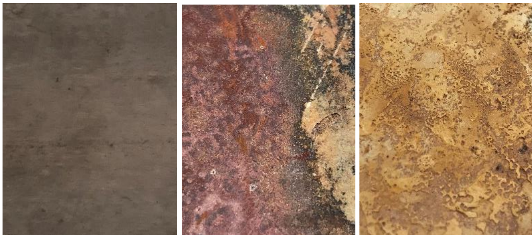
Figure 23: Three stages of steel (no corrosion, mid-corrosion, late corrosion)
