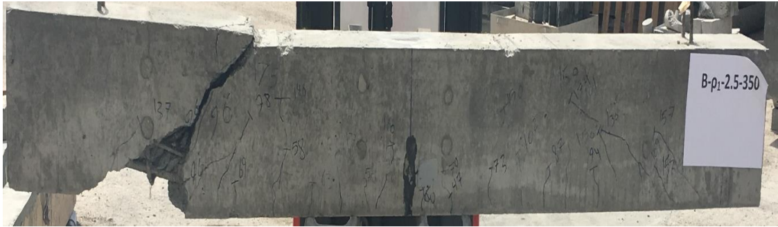
Figure 31. B-2 Diagonal tension failure.
