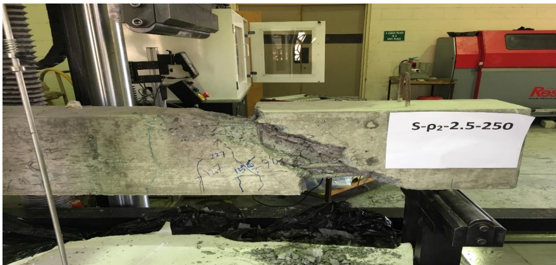
Figure 46. Crushing of the concrete located at the diagonal crack.
