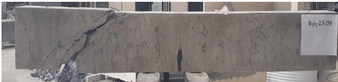
Figure 38. Beam B-6 Diagonal tension failure.
