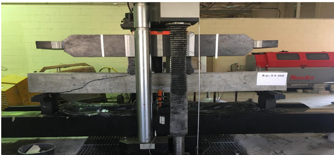
Figure 33. Beam B-3 Diagonal tension failure.
