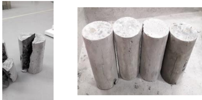
Figure 25. Compressive strength test for the cylinders.
