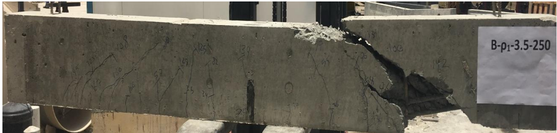
Figure 34. Beam B-4 Shear compression failure.
