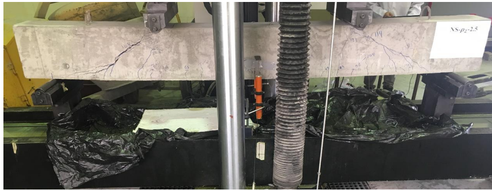
Figure 49. Beam B-13 Diagonal tension failure.
