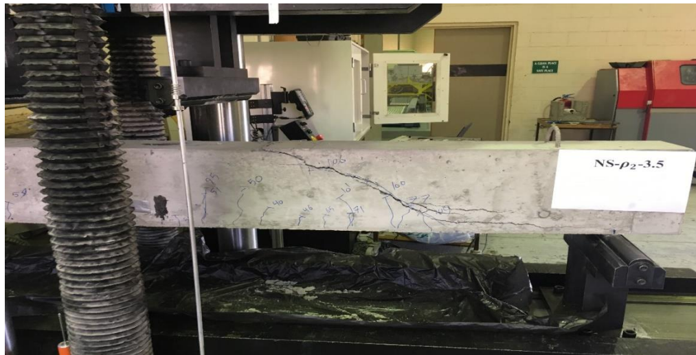
Figure 48. Shear tension failure.
