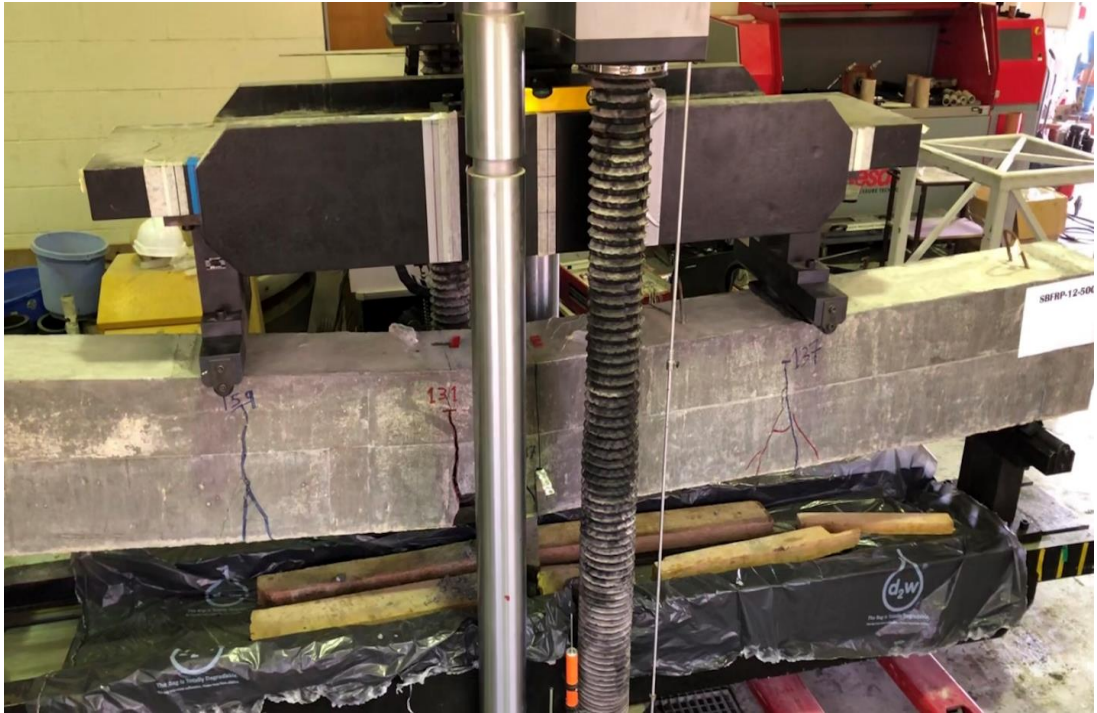
Figure 43: Cracking pattern of beam 4 (SBFRP-12-500)
