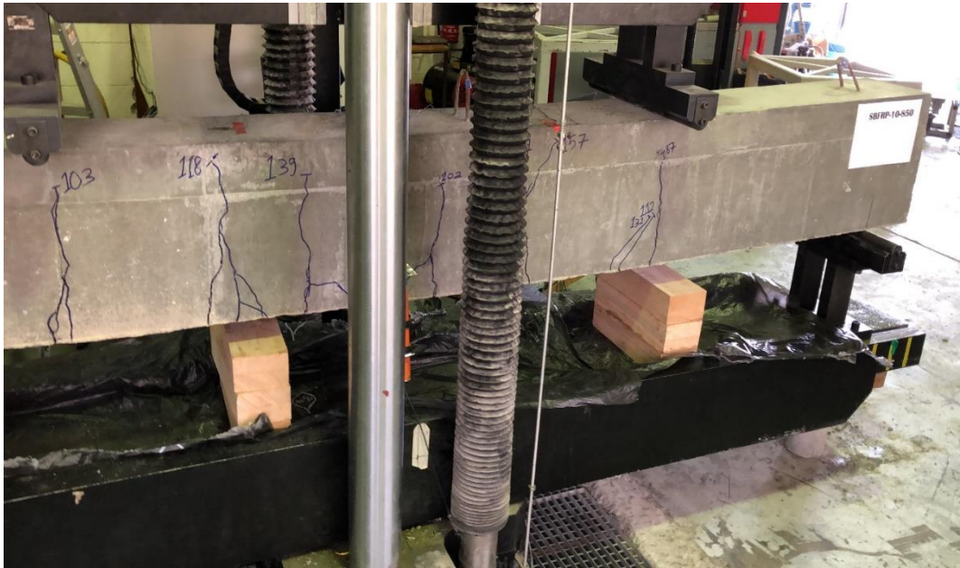
Figure 39: Cracking pattern of beam 3 (SBFRP-10-850)
