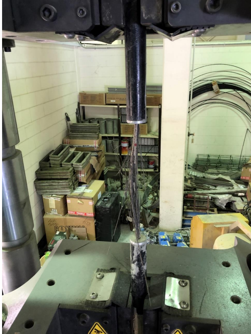
Figure 28: Failure of sand-coated BFRP
