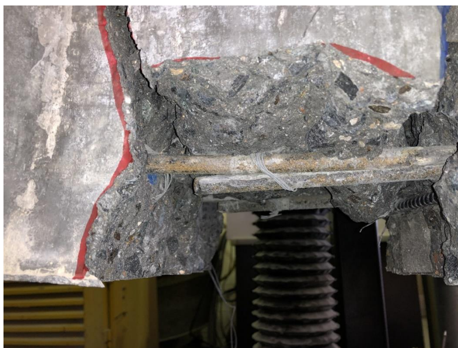
Figure 77: Splitting failure followed by slipping of the FRP bar
