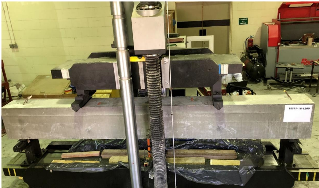
Figure 62: Beam 9 (SBFRP-16-1200) testing setup
