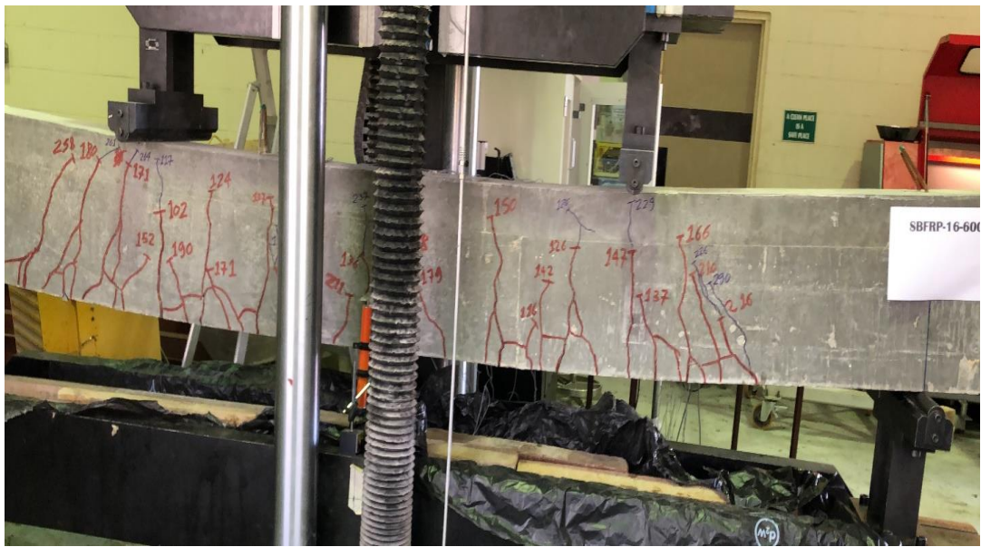
Figure 55: Cracking pattern of beam 7 (SBFRP-16-600)
