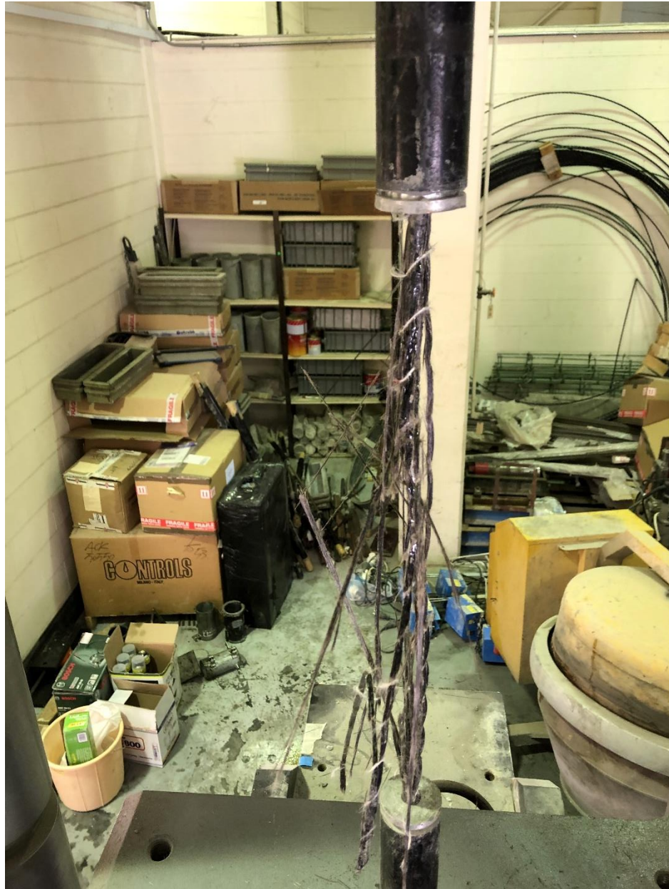
Figure 29: Failure of helically wrapped BFRP
