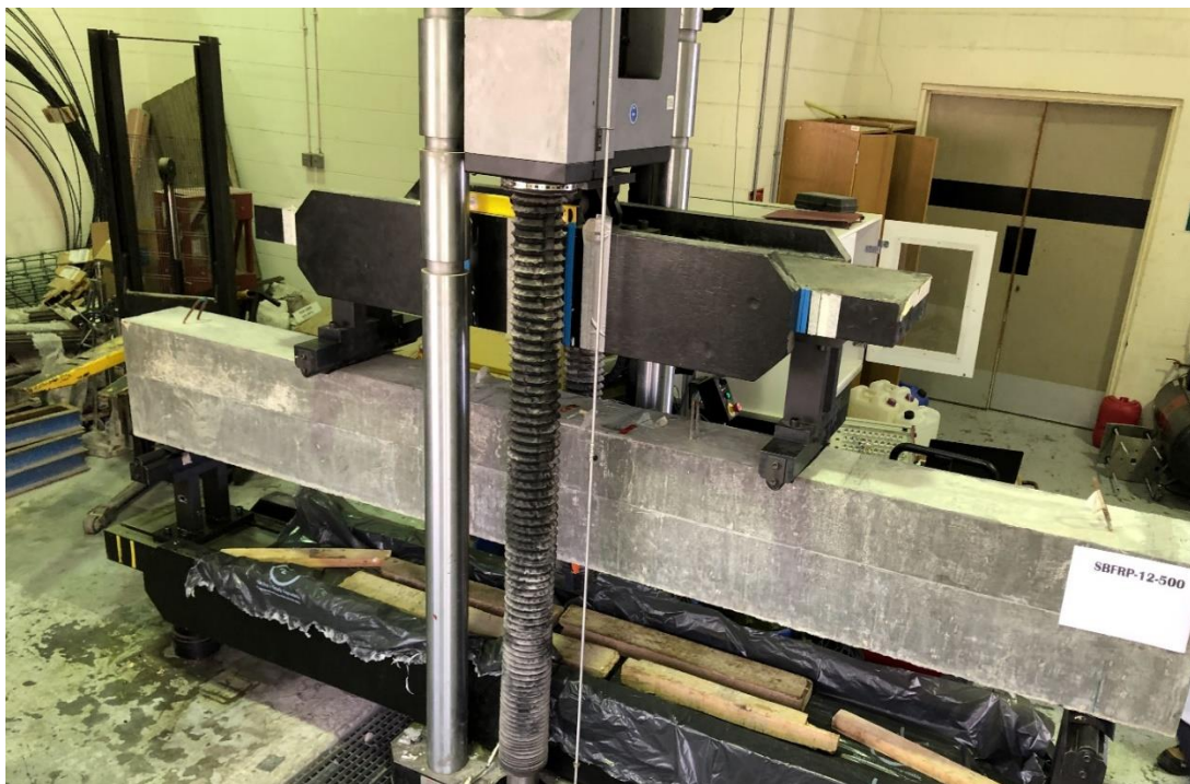
Figure 42: Beam 4 (SBFRP-12-500) testing setup
