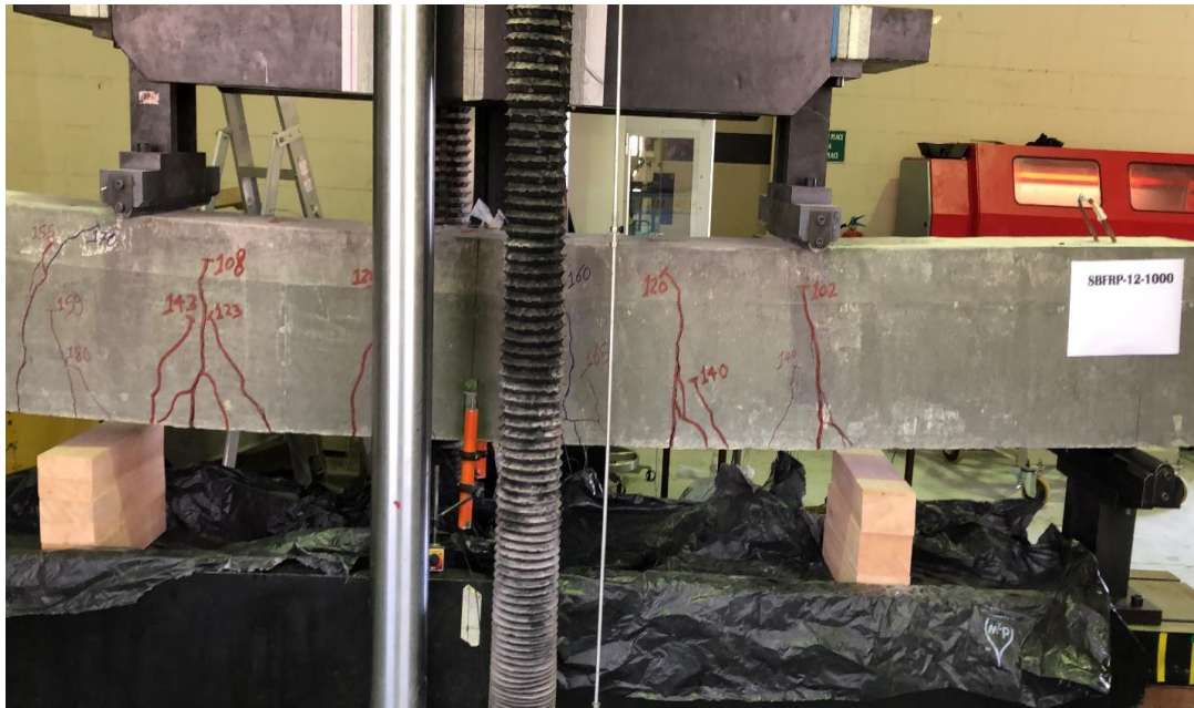
Figure 51: Cracking pattern of beam 6 (SBFRP-12-1000)
