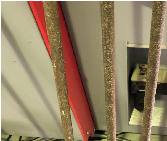
Figure 11: Sand-coated basalt FRP bars
