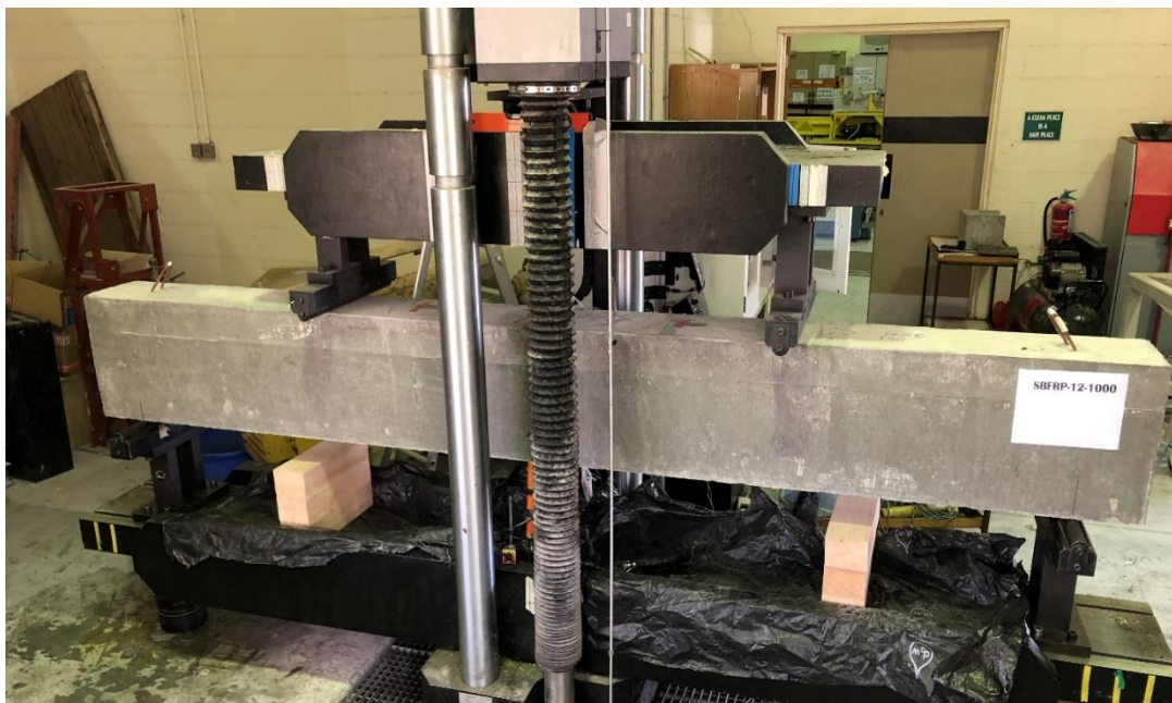
Figure 50: Beam 6 (SBFRP-12-1000) testing setup
