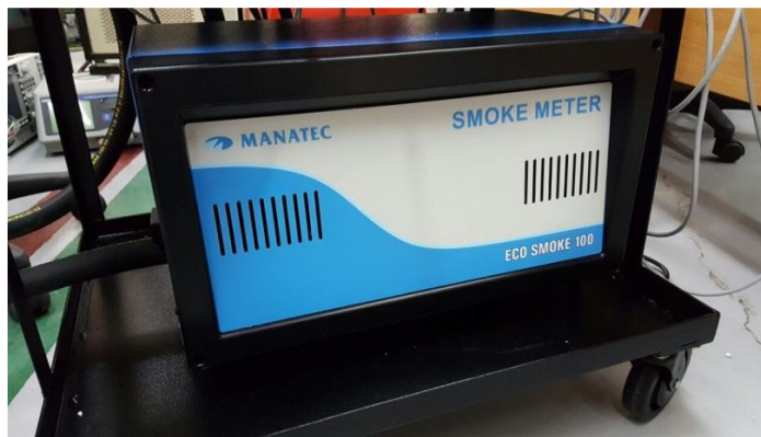
Figure 29. Smoke meter overview
