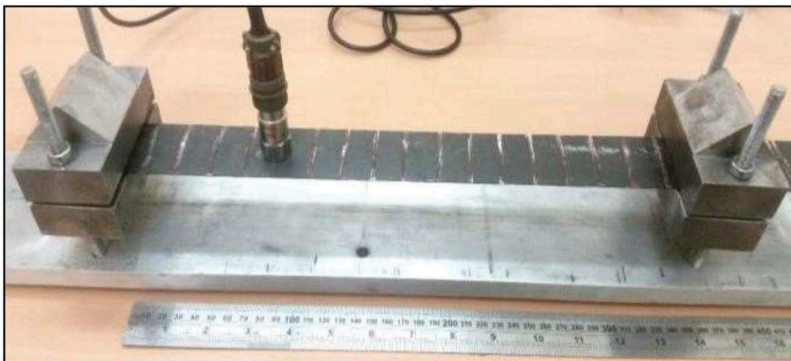
Figure 13. Placement of the accelerometer.
