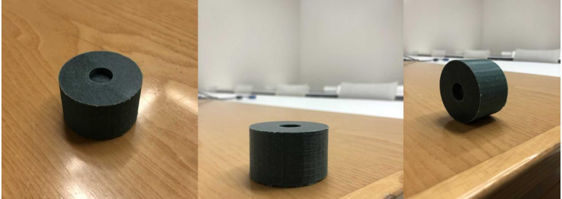
Figure 71. MRE sample after curing.
