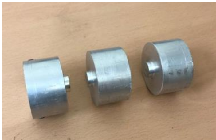
Figure 72. Aluminum coupling parts after manufacturing.
