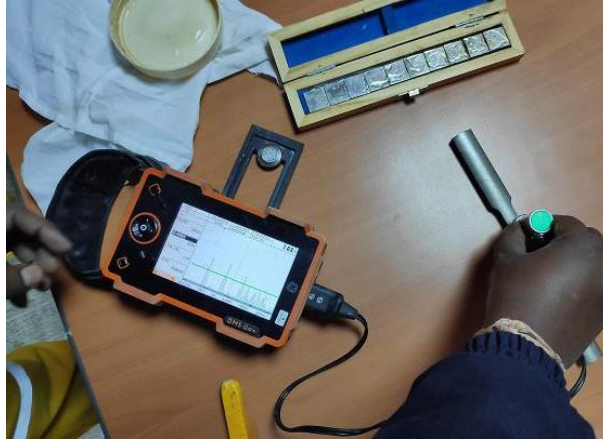
Figure 10. UT measurements for identifying the lowest thickness area in corroded specimens.
