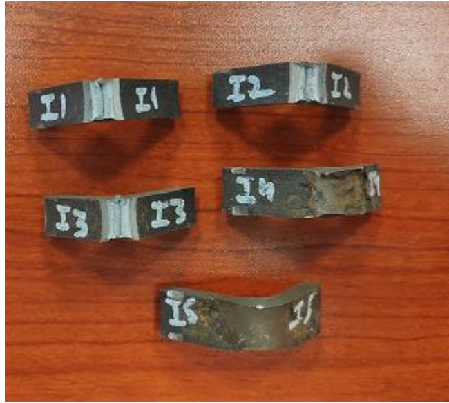
Figure 19. Photograph for the Charpy specimens after the test.
