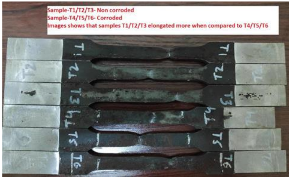
Figure 17. Photograph for the elongated length of all tensile samples after test.
