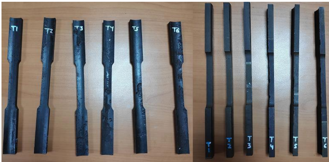
Figure 9. Photograph for the tensile samples (T1-T6).
