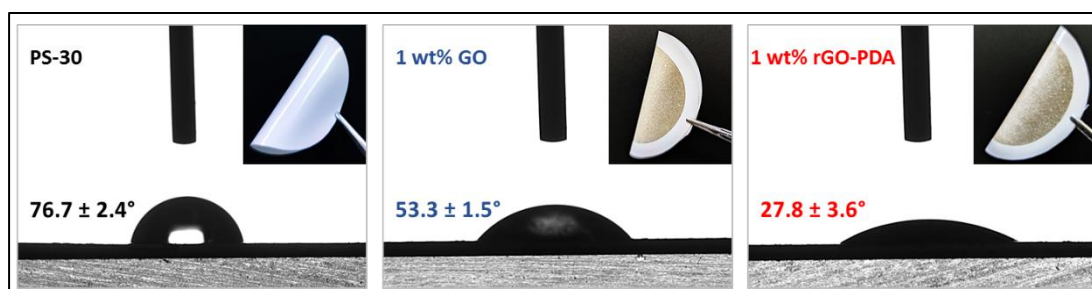
Figure 4-22: Contact angle measurements of the pristine PS-30, PS/GO, and PS/rGO-PDA membranes.
