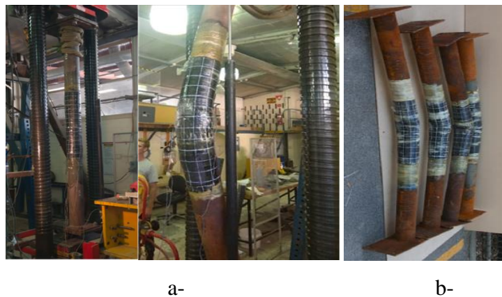
Figure 12. Repaired specimens (a) while and (b) after combined axial compression and bending testing [50].
