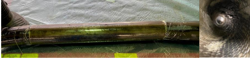
Figure 75. Steps of fabricating the internal reinforcement layer.
