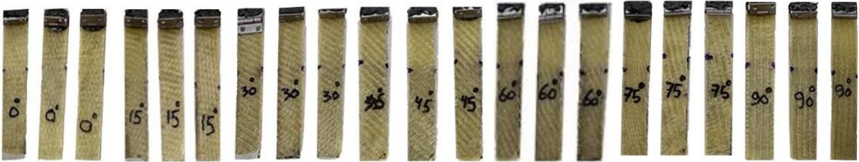
Figure 42. Specimens with different fiber orientation angles for mode I test.
