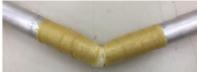
Figure 6. failure of AFRP joining after 3-point bending test[32].
