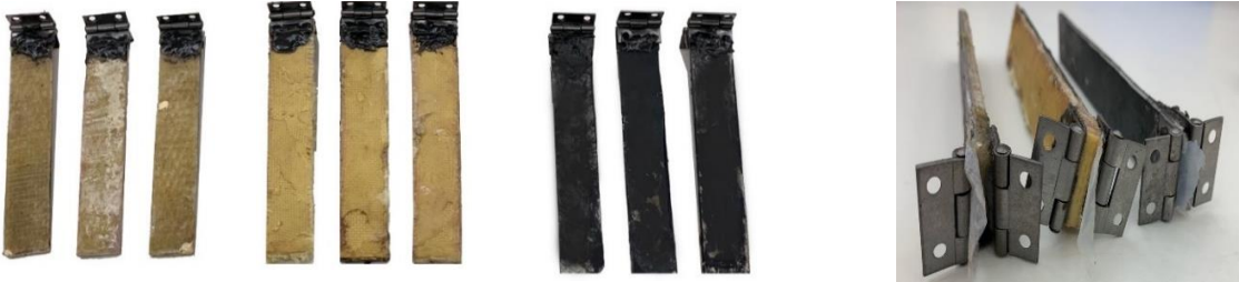
GFRP KFRP CFRP Specimens with PTFE Teflon sheet and hinges
