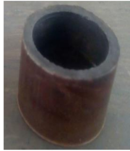
Figure 7. Banana stem reinforced PVC composite pipe [39].
