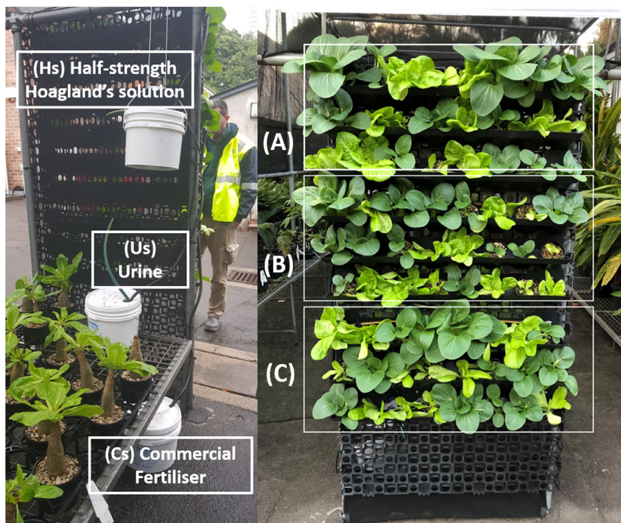
Fig. 6. Picture of the GSky Versa Wall set up with the different growing media. The first three rows (A) were fertilised with Half-strength Hoagland's solution (Hs), the second three (B) with urine (Us) and the bottom three (C) with the commercial nutrients solution (Cs).
