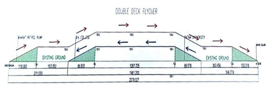
Fig. 3: Sectional Elevation of Double decker flyover on Ashok Rajpath
