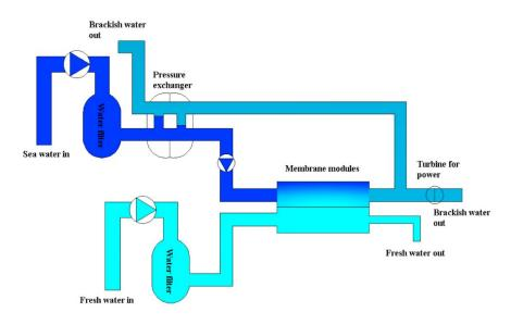
Fig. 4: Process outline for a standard osmotic power plant
