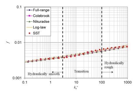
Fig. 6: Friction factor for an open channel
