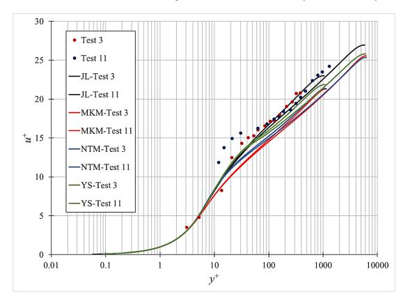
Fig. 1: Comparison of the velocity profiles between model predictions and experimental data by (Kirkgoz, 1989)
