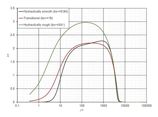
Fig. 5: Turbulent kinetic energy profiles in a rough-bed open channel by SST k- $\omega$  model
