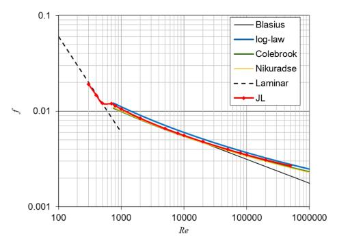
Fig. 2: Friction factor for smooth-bed open channel
