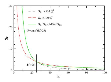
Fig. 3: Model parameter  $S_R$  in k- $\omega$  model to describe bed roughness
