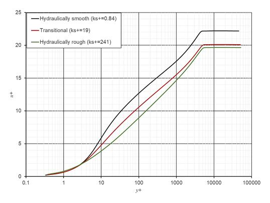
Fig. 4: Velocity profiles in a rough-bed open channel by SST k- $\omega$  model
