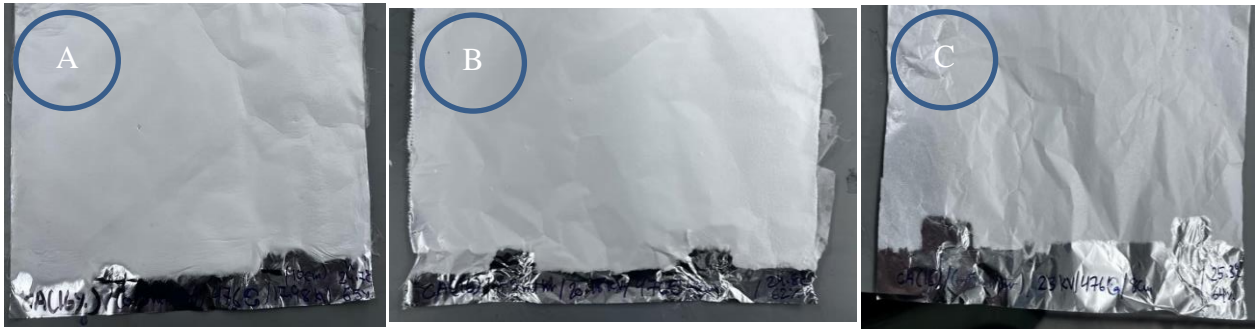
Figuer13: Actual image of Cellulose acetate nanofiber with different applied voltage. (A) 17.89 Kv/ (B) 20 KV / (C) 23 KV.
