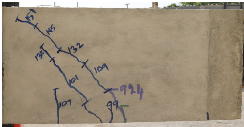
a) Critical shear span
