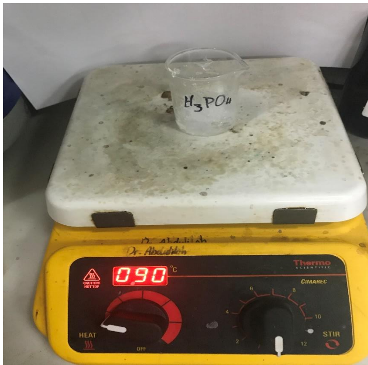
Figure 13. PVA-H 3 PO 4 gel preparation
