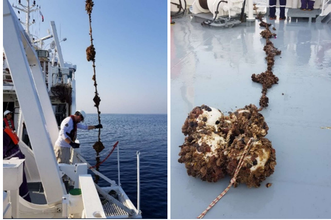
Figure 4. Retrieval of fouling plates onboard the RV Janan; detail of crane operation (left) and trawl floats used to support the structure (right).
