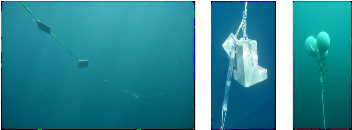
Figure 2. Mooring line (left) supported by two concrete anchors and one acoustic release unit (middle) and; 4x14 L trawl floats (right).
