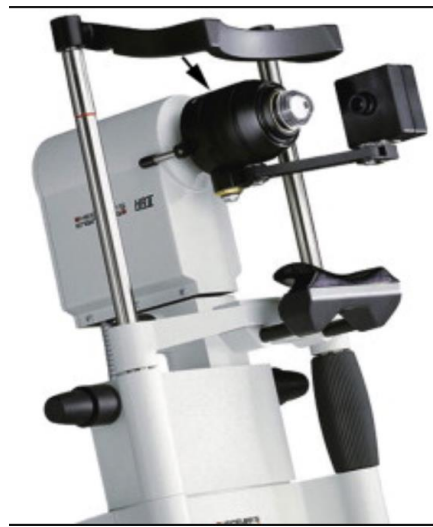
Figure 2. Corneal Confocal Microscope. (The Rostock corneal module is pointed to by the arrow)
