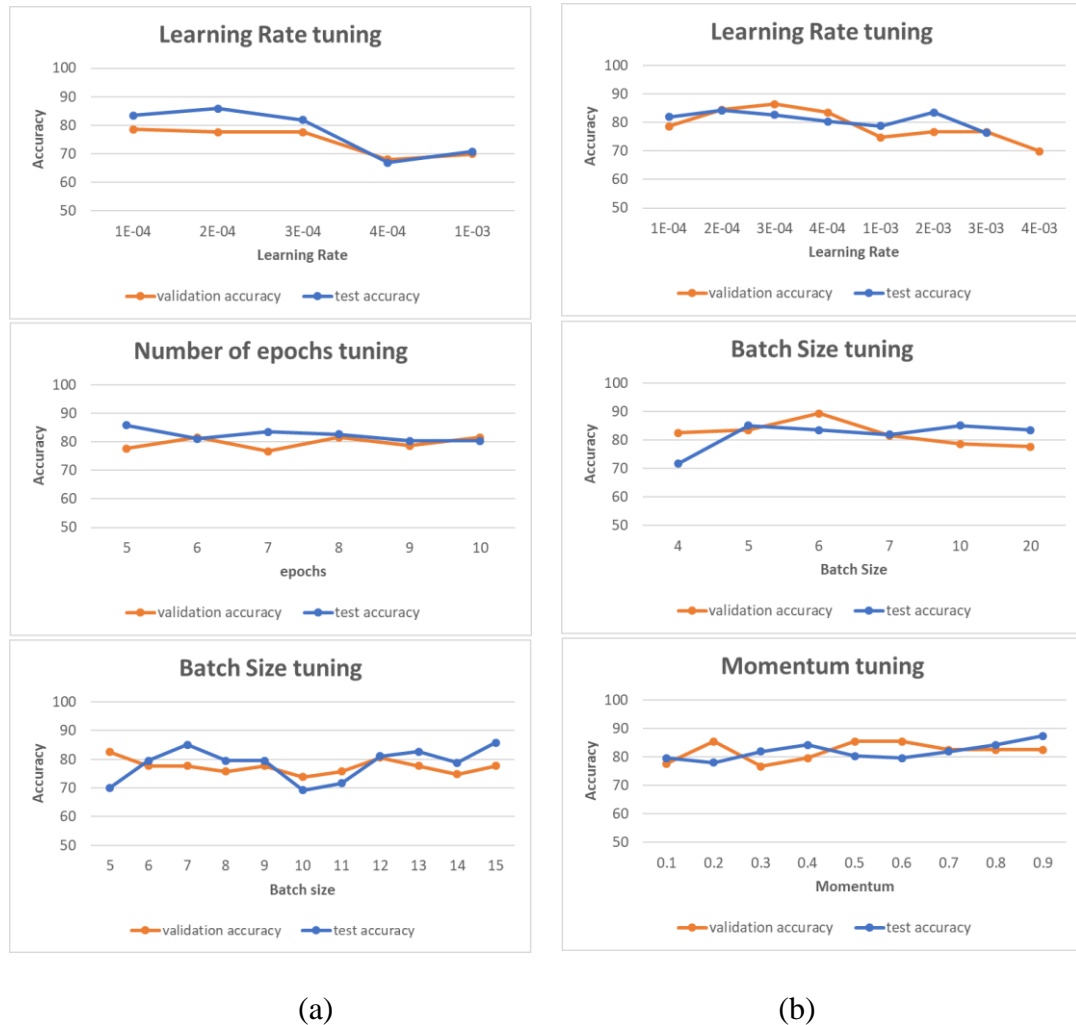
Figure 19. GoogleNet tuning graphs. (a) tuning using the RMSProp solver, (b) tuning using the SGDM solver.
