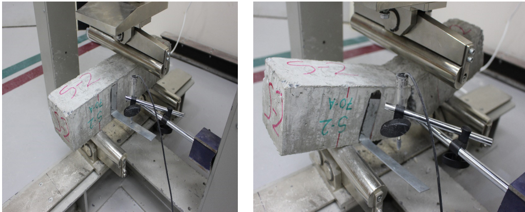
(a) Figure 2: Three-point flexural test (b)
