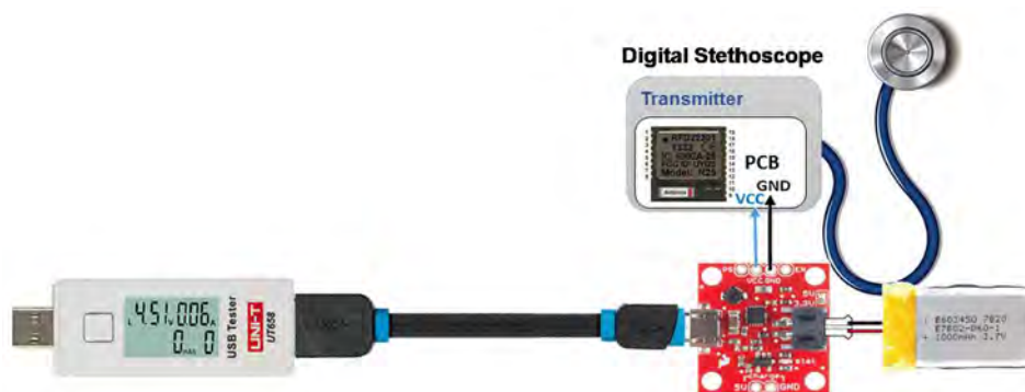
Figure 9. Evaluation of overall power consumption of the sensor module.
