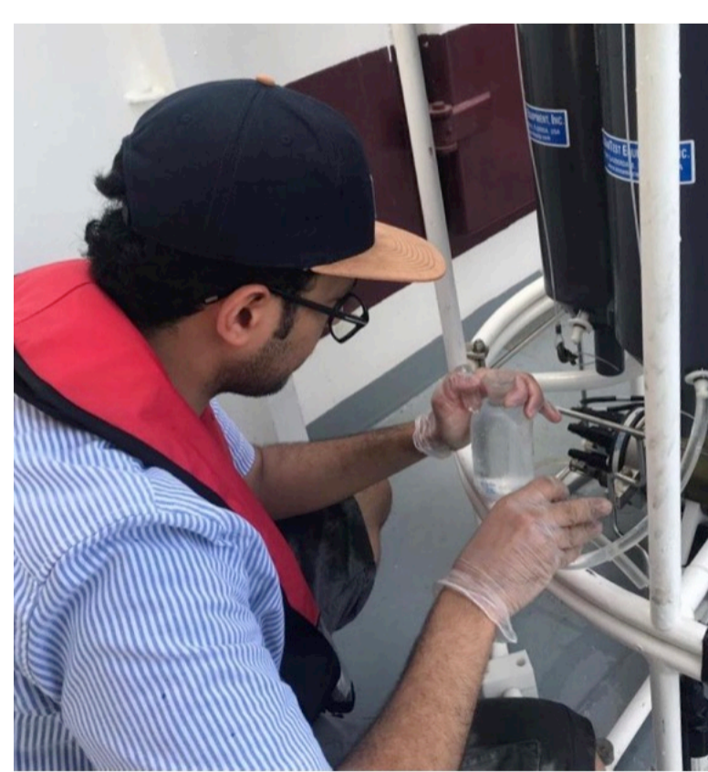
Sampling Seawater for DIC/Alkalinity
