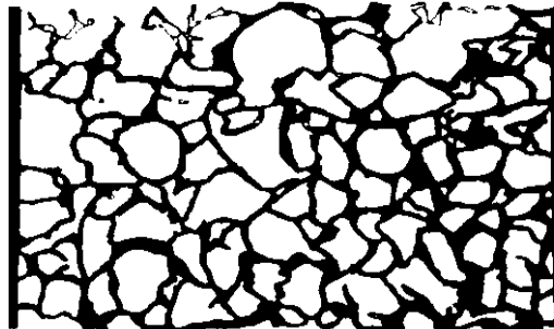
Figure 55. Micromodel after the injection of oil and formation water indicating the residual water.
