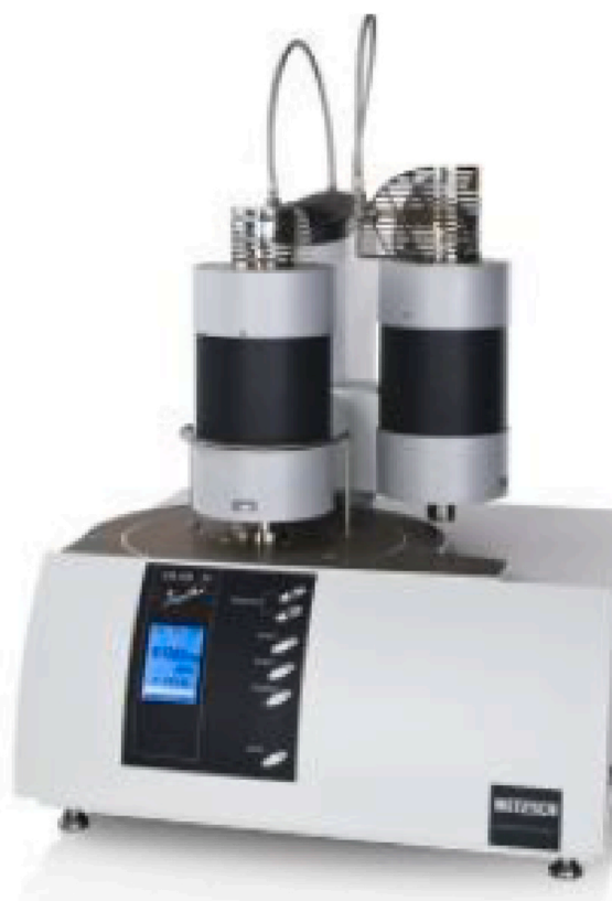
Fig. 4. DSC set up for thermal analysis of the specimen DSC test is done on NETZSCH STA 449F3 in the range of 30 °C–550 °C as shown in Fig. 4. Dynamic scanning is done by increasing the temperature of the prepared sample at the rate of 10 °C/min. Dynamic scans are performed to come up with the average of the total heat of reaction values. The sample size taken for the analysis is 3.3 \pm 1 mg [1].
