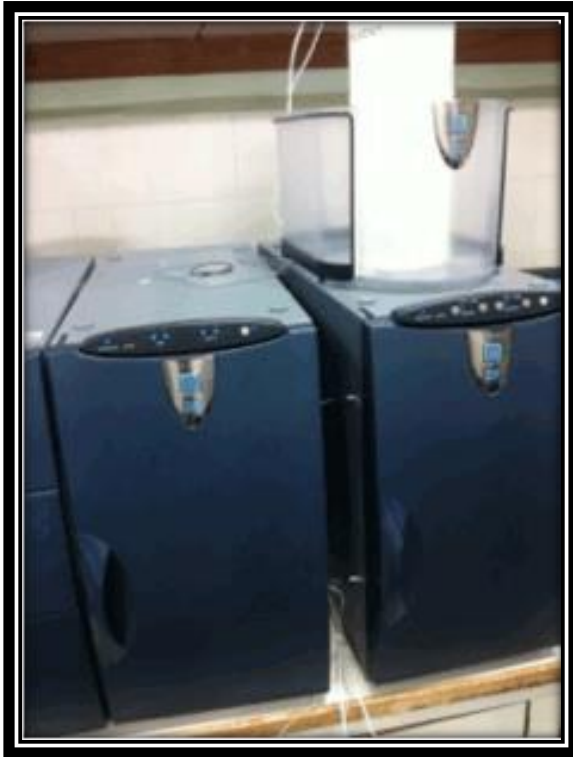
Dionex ICS 5000, used to analyse chlorite, chlorate, and bromate
