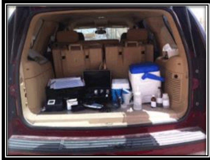
Vehicle used as mini lab and for transportation samples
