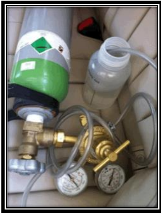
Nitrogen Gas Cylinder used for purging
