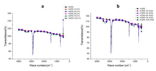
Figure 10. FTIR spectrums of (a) HDPE-P3 and (b) HDPE-MG5 composites.
