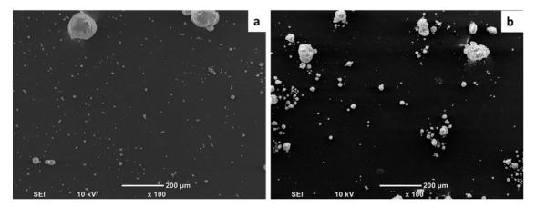
Figure 2. SEM micrographs of the fillers on a conductive adhesive tape: (a) P3; (b) MG5.
