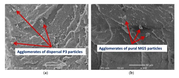
Figure 5. SEM micrographs of the cryo-fractured surfaces of (a) HDPE-10%P3 and (b) HDPE-10%MG5.
