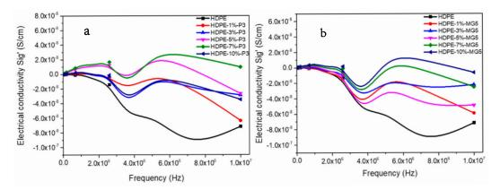
Figure 11. Electrical conductivity-frequency relationship of (a) HDPE-P3 and (b) HDPE-MG5 composites.
