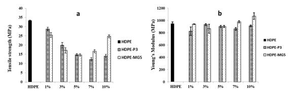
**Figure 6.** Mechanical properties of HDPE-P3 and HDPE-MG5 composites (**a**) tensile strength; (**b**) Young's modulus.
