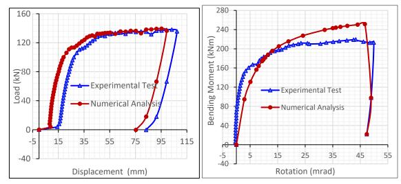
**Fig. 4:** (A) Force – Displacement relationship (B) Moment – Rotation Relationship of composite joint in experimental testing and FE modeling
