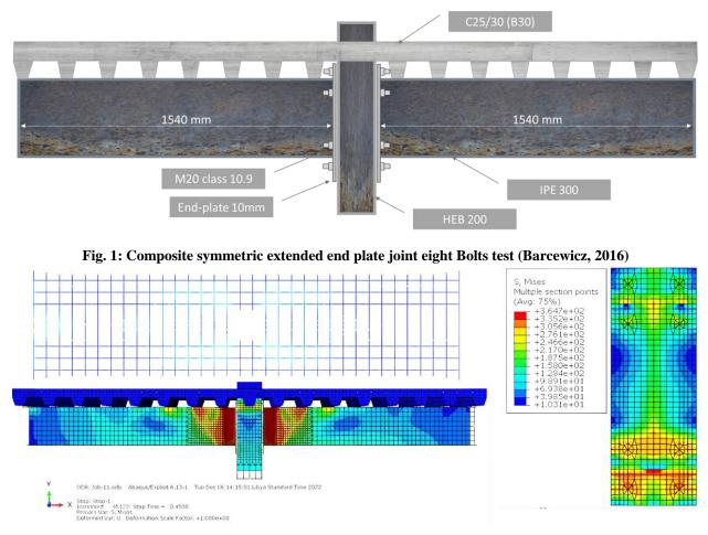
Fig. 2: Displays the stresses in the joint and the overall model using ABAQUS FE modeling
