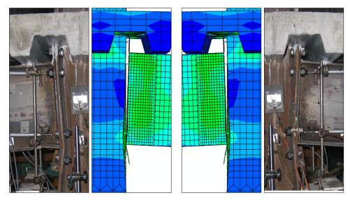
Fig. 3: Joint deformation comparison between experimental testing and FEA modelling
