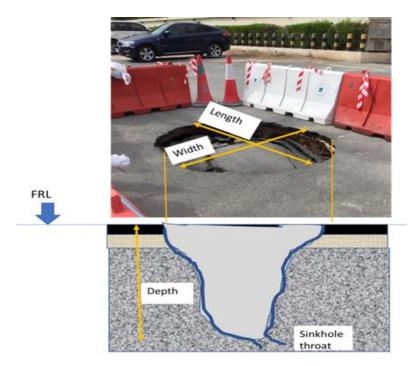
Fig. 3: Measurement of sinkhole dimensions
