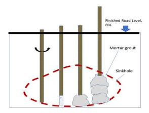
Fig. 5: Schematic diagram of the staged compaction grouting for deep sinkholes
