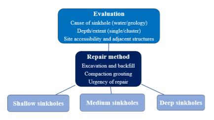
Fig. 2: Sinkhole Repair Methodology
