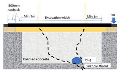
Fig. 4: Schematic diagram of the excavation and backfill repair method
