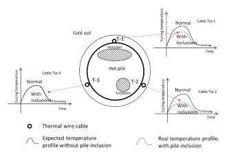
Fig. 5: Conceptual relationship between temperature development and pile integrity
