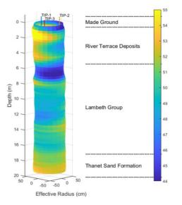
Fig. 4: Predicted pile 3D shape
