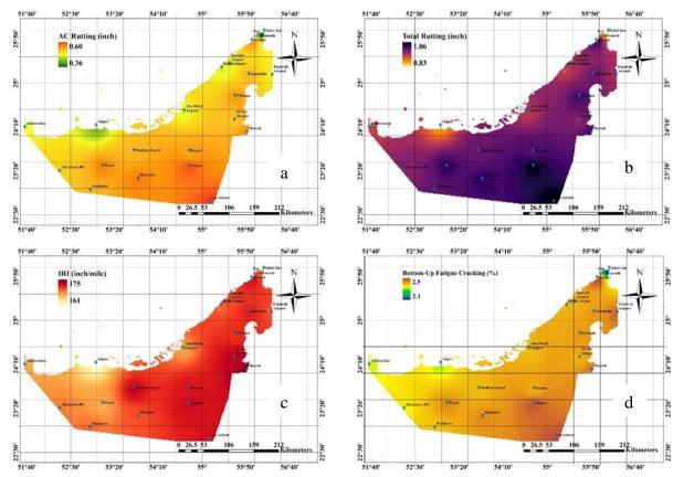
Fig. 3: Simulated (a) AC Rutting; (b) Total Rutting; (c) Terminal IRI; and Bottom-Up Fatigue Cracking Maps
